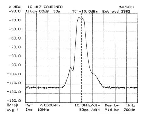
The result of the bandwidth improvement is the reduction of close in intermodulation from multiple signals. The IMD dynamic range will be improved up to 20 dB for signal spacings from 2 to 20 kHz. Also, the blocking dynamic range will be improved for close in signals.
